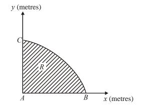
The diagram above shows a cross-section *R* of a dam. The line *AC* is the vertical face of the dam, *AB* is the horizontal base and the curve *BC* is the profile. Taking *x* and *y* to be the horizontal and vertical axes, then *A*, *B* and *C* have coordinates (0, 0),  $(3\pi^2, 0)$  and (0, 30) respectively. The area of the cross-section is to be calculated.
